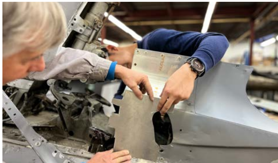
Gene Manchur and Sanni Lapitan affix a replacement section to the aircraft's tail
